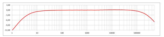
Bandwidth for various Rgen R load=100K //50pF, secondary grounded
